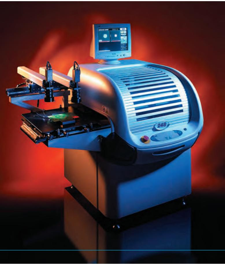
The casting and machine tool bearings used in the 248 ensure accuracy and repeatability for demanding fine pitch applications. Features include: micro controlled set-up and operation; motorised squeegee drive; programmable PCB/stencil separation; and a double squeegee with single pressure setting and independent control of front and rear blades.
