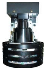
Imaging unit equipped with a telecentric lens
